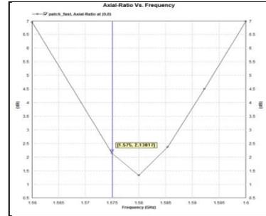
Fig.11.Axial ratio Vs Frequency
