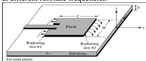
Fig.1. Microstrip Antenna
