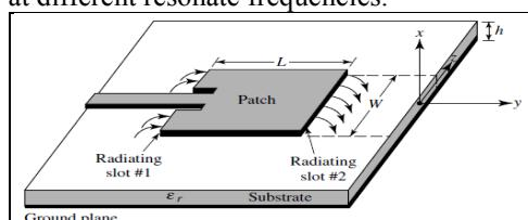
Fig.1. Microstrip Antenna
