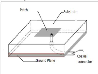
Fig.4. Coaxial Probe Feed
