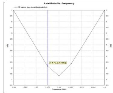
Fig.11.Axial ratio Vs Frequency
