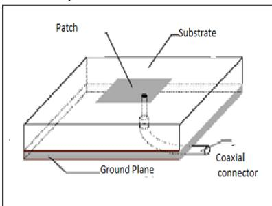
Fig.4. Coaxial Probe Feed
