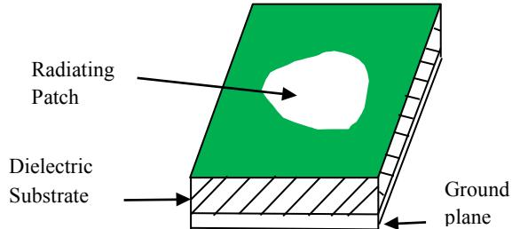
Fig.2. Microstrip antenna configuration
