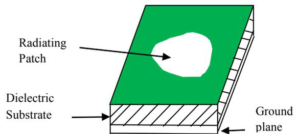
Fig.2. Microstrip antenna configuration
