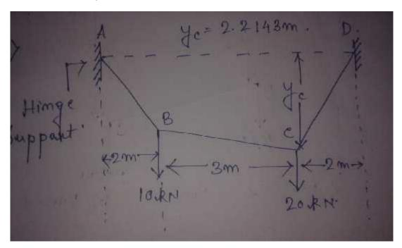
**2.** The total length of a cable system is given as 8.634. Analyze the cable to find the sag at C, and the horizontal tension H.
